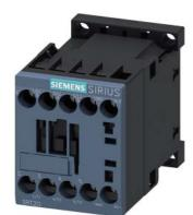
power contactor, AC-3e/AC-3, 9 A, 4 kW / 400 V, 3-pole, 24 V DC, 0.7-1.25\* Us, with integrated diode, auxiliary contacts: 1 NO, screw terminal, size: S00, suitable for PLC outputs, not expandable with auxiliary switch
