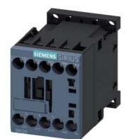
power contactor, AC-3e/AC-3, 9 A, 4 kW / 400 V, 3-pole, 24 V DC, with integrated diode, auxiliary contacts: 1 NO, screw terminal, size: S00  $\,$
