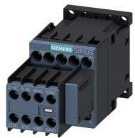
power contactor, AC-3e/AC-3, 9 A, 4 kW / 400 V, 3-pole, 240 V AC, 50/60 Hz, with varistor plugged on, auxiliary contacts: 3 NO + 2 NC, screw terminal, size: S00, removable auxiliary switch
