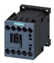
power contactor, AC-3e/AC-3, 9 A, 4 kW / 400 V, 3-pole, 24 V DC, auxiliary contacts: 1 NC, screw terminal, size: S00, upright mounting position
