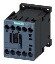
power contactor, AC-3e/AC-3, 9 A, 4 kW / 400 V, 3-pole, 24 V DC, auxiliary contacts: 1 NC, screw terminal, size: S00, communication-capable
