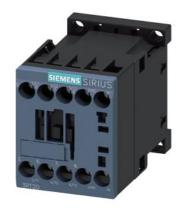
power contactor, AC-3e/AC-3, 9 A, 4 kW / 400 V, 3-pole, 110 V AC, 50 Hz / 120 V, 60 Hz, auxiliary contacts: 1 NC, screw terminal, size: S00, upright mounting position
