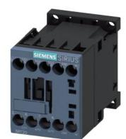
power contactor, AC-3e/AC-3, 9 A, 4 kW / 400 V, 3-pole, 120 V AC, 50/60 Hz, auxiliary contacts: 1 NC, screw terminal, size: S00
