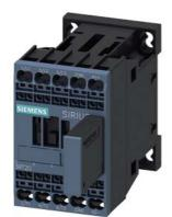
power contactor, AC-3e/AC-3, 7 A, 3 kW / 400 V, 3-pole, 24 V DC, 0.85-1.85\* Us, with varistor plugged on, auxiliary contacts: 1 NC, spring-loaded terminal, size: S00, not expandable with auxiliary switch
