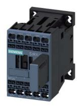
power contactor, AC-3e/AC-3, 7 A, 3 kW / 400 V, 3-pole, 24 V DC, 0.85-1.85 $^{\star}$  Us, with varistor plugged on, auxiliary contacts: 1 NO, spring-loaded terminal, size: S00, not expandable with auxiliary switch
