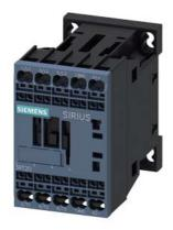
power contactor, AC-3e/AC-3, 7 A, 3 kW / 400 V, 3-pole, 24 V DC, 0.85-1.85\* Us, with integrated diode, auxiliary contacts: 1 NO, spring-loaded terminal, size: S00, not expandable with auxiliary switch
