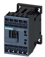
power contactor, AC-3e/AC-3, 7 A, 3 kW / 400 V, 3-pole, 24 V DC, 0.85-1.85\* Us, with integrated suppressor diode, auxiliary contacts: 1 NC, spring-loaded terminal, size: S00
