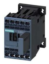
power contactor, AC-3e/AC-3, 7 A, 3 kW / 400 V, 3-pole, 24 V DC, 0.7-1.25\* Us, with varistor plugged on, auxiliary contacts: 1 NO, spring-loaded terminal, size: S00, not expandable with auxiliary switch
