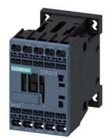
power contactor, AC-3e/AC-3, 7 A, 3 kW / 400 V, 3-pole, 24 V DC, 0.85-1.85\* Us, auxiliary contacts: 1 NC, spring-loaded terminal, size: S00, not expandable with auxiliary switch
