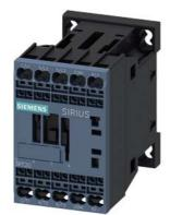
power contactor, AC-3e/AC-3, 7 A, 3 kW / 400 V, 3-pole, 24 V DC, 0.7-1.25\* Us, with integrated diode, auxiliary contacts: 1 NC, spring-loaded terminal, size: S00, suitable for PLC outputs, not expandable with auxiliary switch
