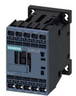
power contactor, AC-3e/AC-3, 7 A, 3 kW / 400 V, 3-pole, 24 V DC, 0.7-1.25\* Us, with integrated diode, auxiliary contacts: 1 NO, spring-loaded terminal, size: S00, suitable for PLC outputs, not expandable with auxiliary switch
