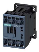
power contactor, AC-3e/AC-3, 7 A, 3 kW / 400 V, 3-pole, 24 V DC, 0.7-1.25\* Us, auxiliary contacts: 1 NC, spring-loaded terminal, size: S00, suitable for PLC outputs, not expandable with auxiliary switch
