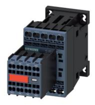
power contactor, AC-3e/AC-3, 7 A, 3 kW / 400 V, 3-pole, 24 V DC, with integrated diode, auxiliary contacts: 2 NO + 2 NC, spring-loaded terminal, size: S00, captive auxiliary switch
