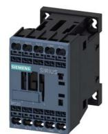
power contactor, AC-3e/AC-3, 7 A, 3 kW / 400 V, 3-pole, 24 V DC, with integrated diode, auxiliary contacts: 1 NO, spring-loaded terminal, size: S00
