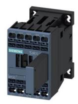
power contactor, AC-3e/AC-3, 7 A, 3 kW / 400 V, 3-pole, 110 V AC, 50 Hz / 120 V, 60 Hz, with plugged-on RC element, auxiliary contacts: 1 NO, spring-loaded terminal, size: S00
