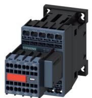
power contactor, AC-3e/AC-3, 7 A, 3 kW / 400 V, 3-pole, 230 V AC, 50/60 Hz, with varistor plugged on, auxiliary contacts: 2 NO + 2 NC, spring-loaded terminal, size: S00, captive auxiliary switch
