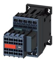
power contactor, AC-3e/AC-3, 7 A, 3 kW / 400 V, 3-pole, 110 V AC, 50 Hz / 120 V, 60 Hz, with varistor plugged on, auxiliary contacts: 2 NO + 2 NC, spring-loaded terminal, size: S00, captive auxiliary switch
