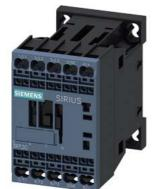
power contactor, AC-3e/AC-3, 7 A, 3 kW / 400 V, 3-pole, 48 V DC, auxiliary contacts: 1 NC, spring-loaded terminal, size: S00,
