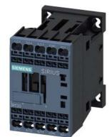
power contactor, AC-3e/AC-3, 7 A, 3 kW / 400 V, 3-pole, 220 V DC, auxiliary contacts: 1 NC, spring-loaded terminal, size: S00,
