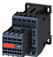
power contactor, AC-3e/AC-3, 7 A, 3 kW / 400 V, 3-pole, 24 V DC, auxiliary contacts: 2 NO + 2 NC, spring-loaded terminal, size: S00, captive auxiliary switch
