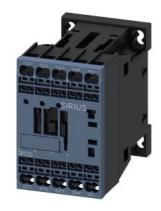
power contactor, AC-3e/AC-3, 7 A, 3 kW / 400 V, 3-pole, 24 V DC, auxiliary contacts: 1 NC, spring-loaded terminal, size: S00, communication-capable
