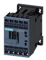
power contactor, AC-3e/AC-3, 7 A, 3 kW / 400 V, 3-pole, 400 V AC, 50/60 Hz, auxiliary contacts: 1 NC, spring-loaded terminal, size: S00  $\,$
