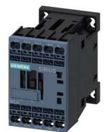
power contactor, AC-3e/AC-3, 7 A, 3 kW / 400 V, 3-pole, 220 V AC, 50 Hz / 240 V, 60 Hz, auxiliary contacts: 1 NO, spring-loaded terminal, size: S00
