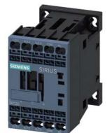
power contactor, AC-3e/AC-3, 7 A, 3 kW / 400 V, 3-pole, 230 V AC, 50/60 Hz, auxiliary contacts: 1 NC, spring-loaded terminal, size: S00
