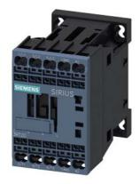
power contactor, AC-3e/AC-3, 7 A, 3 kW / 400 V, 3-pole, 220 V AC, 50/60 Hz, auxiliary contacts: 1 NO, spring-loaded terminal, size: S00  $\,$
