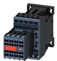
power contactor, AC-3e/AC-3, 7 A, 3 kW / 400 V, 3-pole, 110 V AC, 50 Hz / 120 V, 60 Hz, auxiliary contacts: 2 NO + 2 NC, spring-loaded terminal, size: S00, captive auxiliary switch
