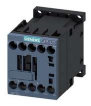
power contactor, AC-3e/AC-3, 7 A, 3 kW / 400 V, 3-pole, 24 V DC, 0.7-1.25\* Us, with integrated suppressor diode, auxiliary contacts: 1 NC, screw terminal, frame size: S00, suitable for PLC outputs, not expandable with auxiliary switch expandable
