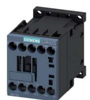
power contactor, AC-3e/AC-3, 7 A, 3 kW / 400 V, 3-pole, 48 V DC, auxiliary contacts: 1 NO, screw terminal, size: S00  $\,$
