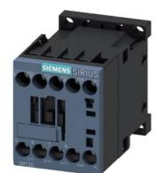
power contactor, AC-3e/AC-3, 7 A, 3 kW / 400 V, 3-pole, 220 V AC, 50 Hz / 240 V, 60 Hz, auxiliary contacts: 1 NC, screw terminal, size: S00  $\,$
