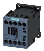
power contactor, AC-3e/AC-3, 7 A, 3 kW / 400 V, 3-pole, 208 V AC, 50/60 Hz, auxiliary contacts: 1 NC, screw terminal, size:  $\rm S00$
