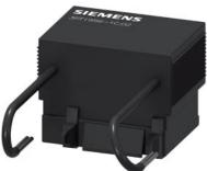
Surge suppressor (RC element) for 3RT1 S6, S10, S12 with spring-type terminal (drive) 400...600 V AC
