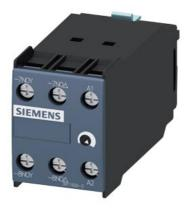
Solid-state time-delayed auxiliary switch, can be snapped on at the front, time range 1.5...30s, 24 V AC/DC, 2 NO, star-delta (wye-delta) function, sizes S6...S12
