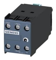
Solid-state time-delayed auxiliary switch, can be snapped on at the front, time range 1.5...30s, 100 ... 127 V AC, 2 NO, star-delta (wye-delta) function, sizes S6...S12
