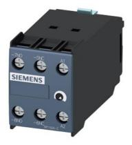
solid-state time-delayed front-side auxiliary switch Time range 0.05...1 s, 200 ... 240 V AC / DC, 1 NO contact, 1 NC contact OFF delay, without control signal for 3RT1
