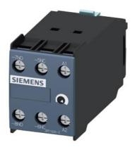
solid-state time-delayed front-side auxiliary switch Time range 0.5...10 s, 100 ... 127 V AC / DC, 1 NO contact, 1 NC contact OFF delay, without control signal for 3RT1
