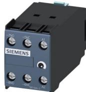
solid-state time-delayed front-side auxiliary switch Time range 0.05...1 s, 100 ... 127 V AC / DC, 1 NO contact, 1 NC contact OFF delay, without control signal for 3RT1
