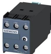
solid-state time-delayed front-side auxiliary switch Time range 5...100 s, 24 V AC/DC, 1 NO contact, 1 NC contact OFF delay, without control signal for 3RT1
