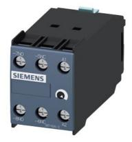
solid-state time-delayed front-side auxiliary switch Time range 0.05...1 s, 24 V AC/DC, 1 NO contact, 1 NC contact ON delay, for 3RT1
