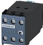
solid-state time-delayed front-side auxiliary switch Time range 5...100 s, 200  $\dots$  240 V AC, 1 NO contact, 1 NC contact ON delay, for 3RT1
