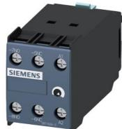
solid-state time-delayed front-side auxiliary switch Time range 0.05...1 s, 100 ... 127 V AC, 1 NO contact, 1 NC contact ON delay, for 3RT1
