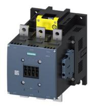
power contactor AC-1 690 A / 690 V / 40  $^{\circ}$ C 3-pole, Uc: 200-277 V AC(50-60 Hz) / DC F-PLC input 24 V DC drive: electronic auxiliary contacts 2 NO + 2 NC main circuit: busbar control and auxiliary circuit: screw terminal
