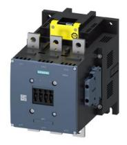
power contactor AC-1 690 A / 690 V / 40  $^{\circ}$ C 3-pole, Uc: 96-127 V AC(50-60 Hz) / DC F-PLC input 24 V DC drive: electronic auxiliary contacts 2 NO + 2 NC main circuit: busbar control and auxiliary circuit: screw terminal
