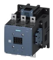
power contactor AC-1 690 A / 690 V / 40  $^{\circ}$ C 3-pole, Uc: 220-240 V AC(50-60 Hz) / DC drive: conventional auxiliary contacts 2 NO + 2 NC main circuit: busbar control and auxiliary circuit: screw terminal
