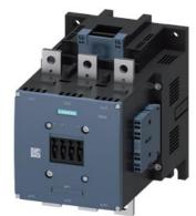
power contactor AC-1 690 A / 690 V / 40  $^\circ$ C 3-pole, Uc: 220-240 V AC(50-60 Hz) / DC drive: conventional auxiliary contacts 2 NO + 2 NC main circuit: busbar control and auxiliary circuit: spring-loaded terminal
