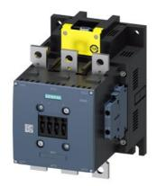
power contactor AC-1 400 A / 690 V / 40  $^{\circ}$ C 3-pole, Uc: 200-277 V AC(50-60 Hz) / DC F-PLC input 24 V DC drive: electronic auxiliary contacts 2 NO + 2 NC main circuit: busbar control and auxiliary circuit: screw terminal
