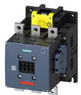
power contactor AC-1 400 A / 690 V / 40 °C 3-pole, Uc: 200-277 V AC(50-60 Hz) / DC F-PLC input 24 V DC drive: electronic auxiliary contacts 2 NO + 2 NC main circuit: busbar control and auxiliary circuit: screw terminal
